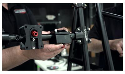
Disassemble rear mounts from packaging, Install the Rear Sliders onto the Seat Rear Support Bar. (This example is NOT sanded) Set Face of Slider flat at 90 deg from bottom housing The system needs to be square in order for the Pistons and **Sliders to move freely** When Slider Flats and Piston Assemblies are at 90 deg. Tightenall bolts one last time. After seat is finally mounted to **Rear Sliders remove Installation** set screw. Bottom screw remains as a safety
