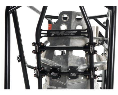
Install Rear Slider Bolts. When System is complete remove Socket Head Allen Set Screw under slider
