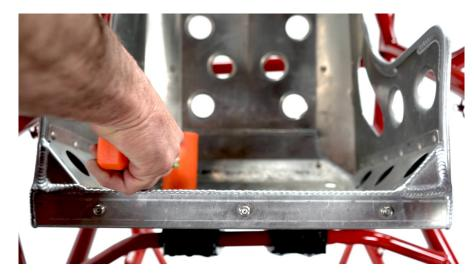
Set Seat in Chassis Start at Piston's for Mounting Seat. Use a Dead Blow Hammer, Hit Seat Bottom to Indent Transfer marks. Remove Seat and Drill 3/8" holes where transfer marks are.
