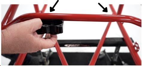
Set Seat in Chassis to verify Mounting Side for Pistons! Use angle finder on Flat bottom of seat to Repeat on Piston Assemblies. (write down angle) Sandwich the bottom housing onto the seat tube CASM logo always is the top, Install both assembly Bodies with bolts and set angle of housing to bottom of seat Angle Typically the center of each Bottom Assembly is Centerline with the Bolt Holes.
