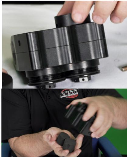
When Assembly is at proper angle on top of body fully Tighten and Insert transfer punch Drop in's into Outside Piston's Only. Inside Pistons are floating Only Tighten all 12 bolts to where the units are Snug to the bar. When bottom assemblies are in final position they should be level with each other side to side, and same angle as Seat Bottom Flat Front to Back
